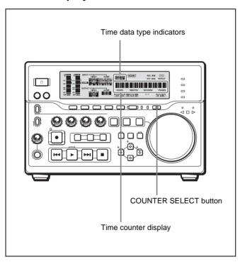
Press the COUNTER SELECT button on the front panel. Each press of this button cycles through three options: CNT value, time code, and user bit data. The time data type indicator for each option lights as it is selected.
